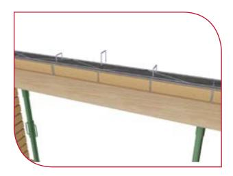
In the vertical joints of the masonry you install **firunc GD** attached always to one of the transverse wires of **firufor**® reinforcement.
