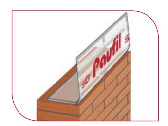
On top of Paufil® put a layer of mortar which provides a strong element for precast concrete. You can also place a layer of neoprene.
