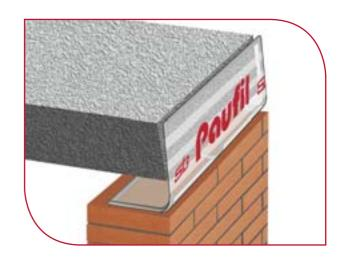
The **Paufil®** formwork should always be at a minimum distance of 2 cm from the inner edge of the enclosure, to prevent possible rust stains on the ceilings.
