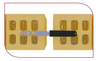
■ In structures where the bricks are more than 12cm it is recommended that the keys in the joints do not exceed the minimum distance of 50cm apart vertically.
